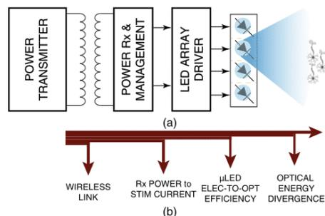
Fig. 1: (a) Top-level block diagram of an implantable optical stimulator with (b) major power losses indicated.
