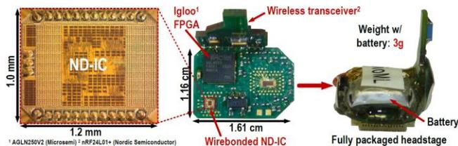
Figure 1: ND-IC (left), headstage (center) and packaged (right).
