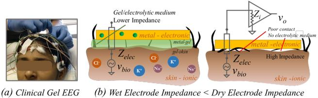
Fig. 1. (a) Typical clinical application of wet electrodes in an EEG clinic (b) Illustration of dry versus wet electrodes on skin.
