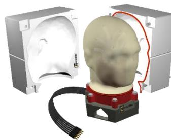
To validate the phantom, human subjects walk on a treadmill in conjunction with a Vicon motion capture system while wearing various COTS gel and dry EEG systems. Motion profiles are then recreated using a 6-dof motion platform with a phantom head model attached, with the phantom wearing the same COTS systems. Additionally EIS with the phantom materials and electrodes provides assessment of the conductive noise and signal transfer.
